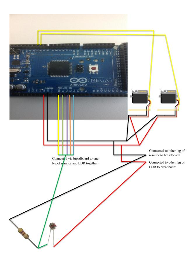
Breadboard not shown, all connections need to be made via breadboard.
